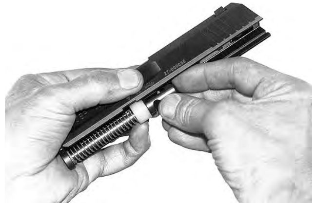
Insert the recoil spring guide rod
